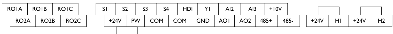
Connection terminal diagram for inverters \geq 4\text{kW}
