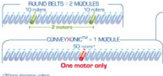
This device is also designed for curved conveyor lines
